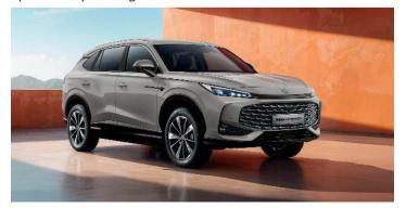
The powertrain consists of a dedicated 1.5T Hybrid petrol engine (105kW), working in conjunction with an electric motor (146kw) powered by an on-board generator and large capacity 1.8kWh battery.
